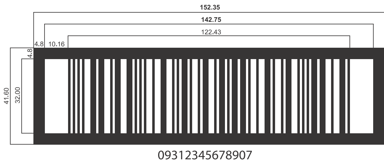
Figure 53 - ITF Bar Code with X-dimension 1.016mm
