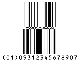
Figure 4 - GS1 DataBar Stacked Omnidirectional Bar Code
