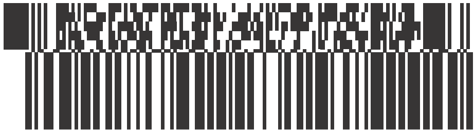
Figure 18 - GS1-128 Composite Symbol with CC-C
