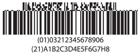
Figure 25 - GS1-128 Symbol with a Four-Column CC-A
