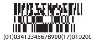
Figure 22 - GS1 DataBar Stacked Symbol with a Two-Column CC-A
