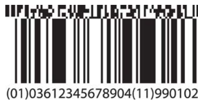
Figure 21 - GS1 DataBar Omnidirectional Symbol with a Four-Column CC-A
