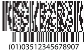
Figure 23 - GS1 DataBar Limited Symbol with a Three-Column CC-B
