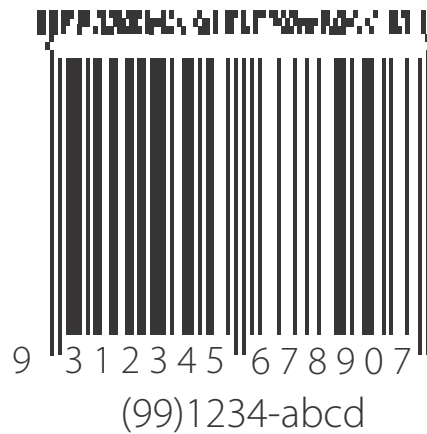
Figure 20 - EAN-13 Symbol with a Four-Column CC-A Component
