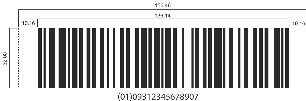
Figure 14 GS1-128 Bar Code at 100%
