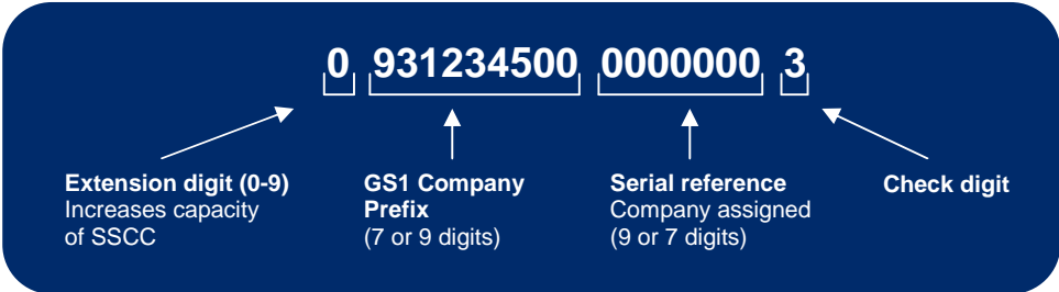
Figure 6: structure of the SSCC
