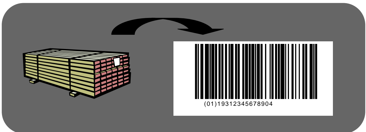
Diagram 36: Example of a standard set length pack of timber allocated a GTIN-14 represented in a GS1-128 Bar Code Symbol
