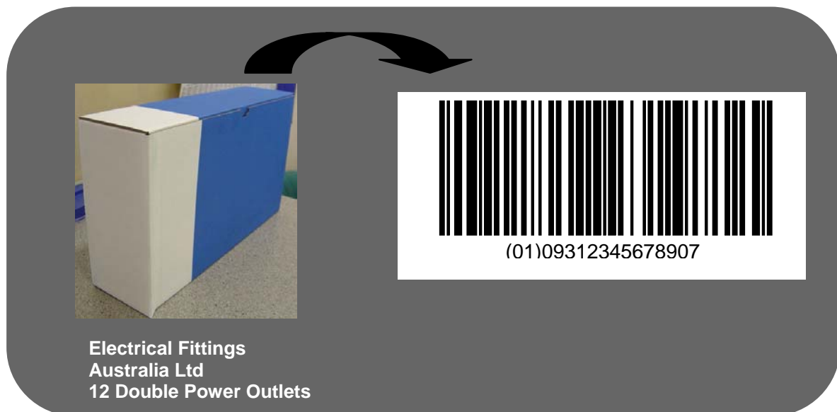
Diagram 58: Example of a carton of double power outlets allocated a GTIN-13 with a filler zero represented in a GS1-128 Bar Code Symbol
