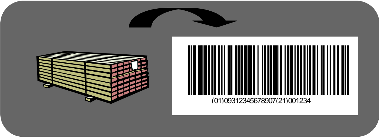
Diagram 44: Pack of Timber representing fixed measure GTIN and serial number in a GS1-128 Bar Code Symbol
