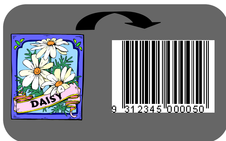
Diagram 19: Example of a packet of daisy seeds allocated a GTIN-13 represented in an EAN-13 Bar Code Symbol
