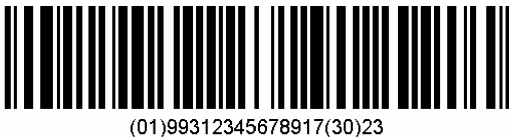
Figure 25: Variable measure GTIN combined with a count of the number of items contained within the non-retail traded unit.
