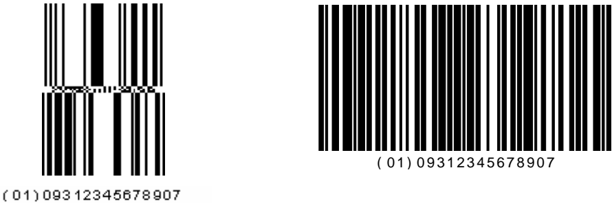
Figure 7: GTIN-13 with a filler zero represented in GS1 DataBar or GS1-128 Bar Code Symbol
