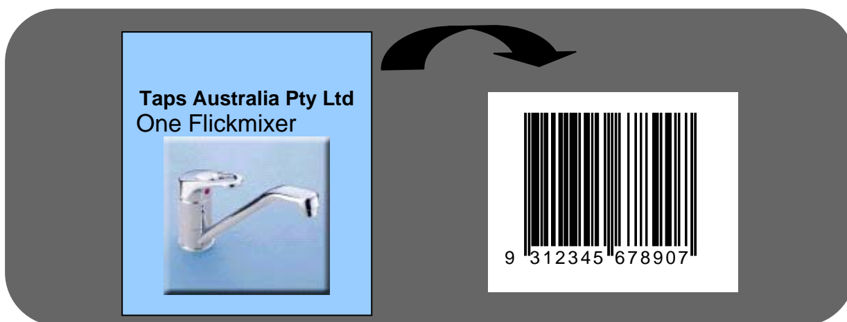
Diagram 45: Example of a tap allocated a GTIN-13 represented in an EAN-13 Bar Code Symbol
