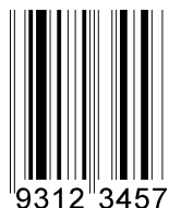
Figure 10: Example of an EAN-8 Bar Code representing the GTIN-8
