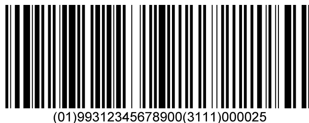
Figure 19: GS1-128 Symbol representing a Variable Measure Trade Item with a length of 2.5 metres
