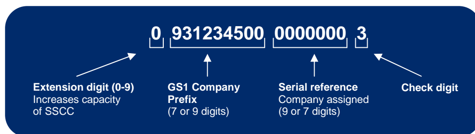
Figure 23: structure of the SSCC
