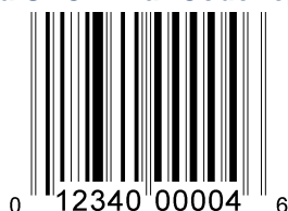
Figure 11: Example of a UPC-A Bar Code representing the GTIN-12
