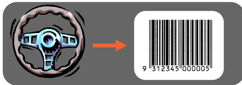
Diagram 10: Example of a trade item carrying an EAN/UCC-13 number represented in an EAN-13 bar code
