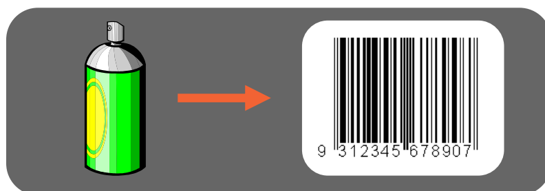
Diagram 9: Example of a trade item carrying an EAN/UCC-13 number represented in an EAN-13 bar code
