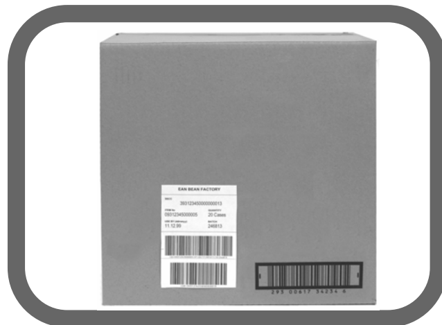
Diagram 19: Location of the EAN•UCC Logistics Label on a carton or unit less than 1 metre in height with the unit already marked with pre-existing bar code
