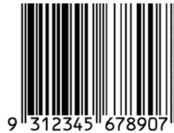
Diagram 10: Example of a trade item carrying an EAN/UCC-13 number represented in an EAN-13 bar code
