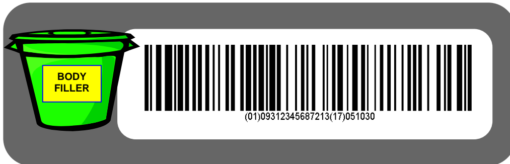
Diagram 5: UCC/EAN 128 Barcode with Expiration Date (Use By)
