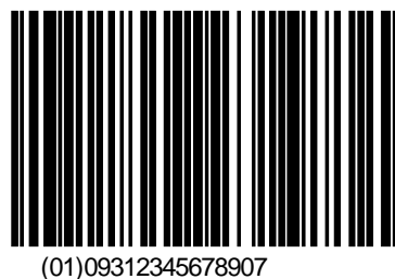
Figure 3: UCC/EAN-128 Bar code
